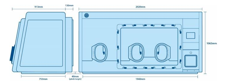
**Important note:** If bench mounted, a further minimum clearance of 500mm is required above the unit and a minimum clearance of 500mm on both sides of the unit is required for user/service access.
